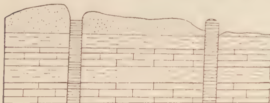
FIG. 321.—Diagram showing the effect of weathering upon two dikes (shown by horizontal lines), one of which is more resistant than the surrounding rock and the other less resistant.
